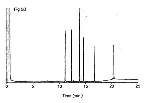
Figure 2 Analysis of polymeradditive test mixture. Comparison of (A) on-column injection and (B) high temperature PTV injection.
