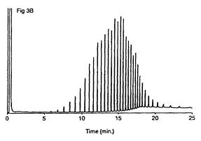
Figure 3. HT-GC separation of Polywax 655. Influence of PTV final temperature. A: final temperature = 400 °C. B: Final temperature = 599 °C. GC temperature programme started at 75 °C.
