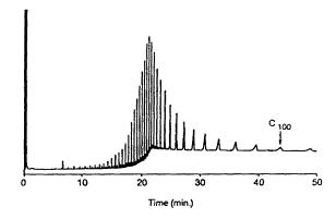
Figure 5. HT-GC separation of Polywax 1000. GC temperature programme started at 75 °C.
