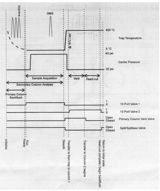
FIGURE 4. Temperature, carrier pressure, and valve events during 2D-GC analysis cycle.
