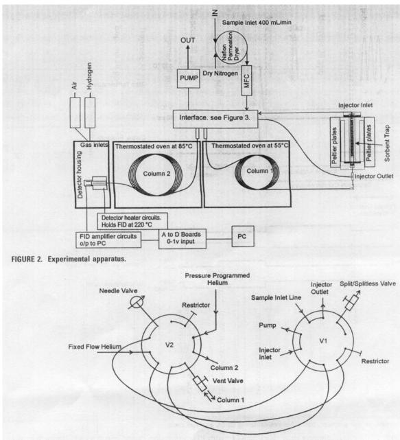
Interface set in sample acquire / secondary column analysis position. V1 position 1, V2 position 0
