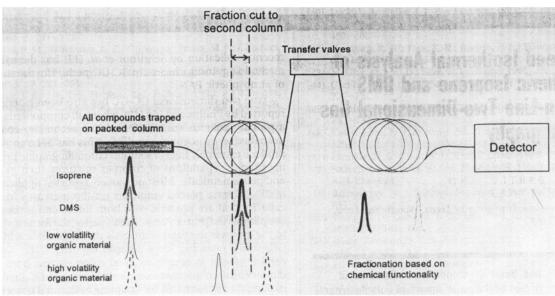
FIGURE 1. Schematic of the PTV-GC-GC separation process.
