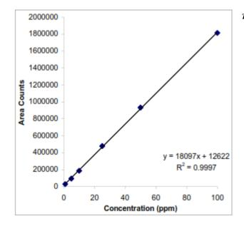
*Figure 2:* Calibration of ethylene glycol, concentration from 1 ppm to 100 ppm
