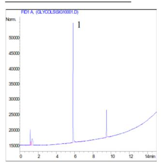
Figure 1: 2uL cold split injection of 5ppm ethylene glycol (1) standard
