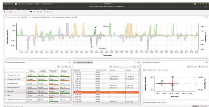
Figure 2: Screenshot of the ChromIdent® software showing the results of a comparison of a polymer mix analysis with a previously created database.
