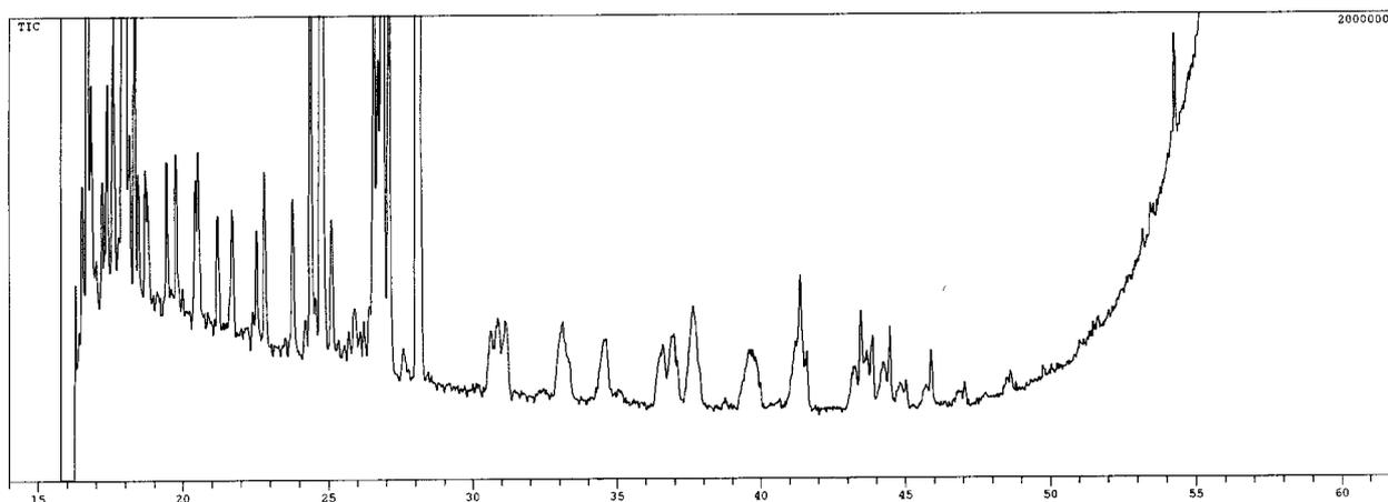
**Figure 5:** On-line SPE–PTV–GC–MS chromatogram of 10 mL of Eindhoven tap water spiked at the level of 1  $\mu\text{g/L}$  using a too short solvent vent time.
