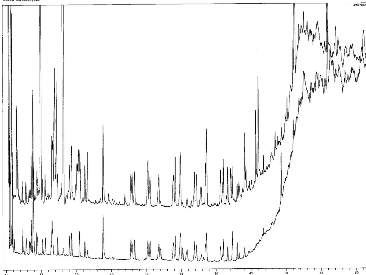
**Figure 3.** Lower chromatogram, 50  $\mu\text{l}$  of an 200  $\text{g}/\mu\text{l}$  standard; Upper chromatogram, Off-line SPE PTV–GC–MS full scan chromatogram of 10 mL spiked Meuse water at the level of 1  $\mu\text{g}/\text{l}$ .
