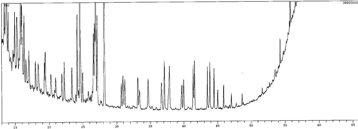
**Figure 6.** On-line SPE-PTV-GC-MS chromatogram of 10 mL of Eindhoven tap water spiked at the level of 1 µg/L using correct solvent vent time.
