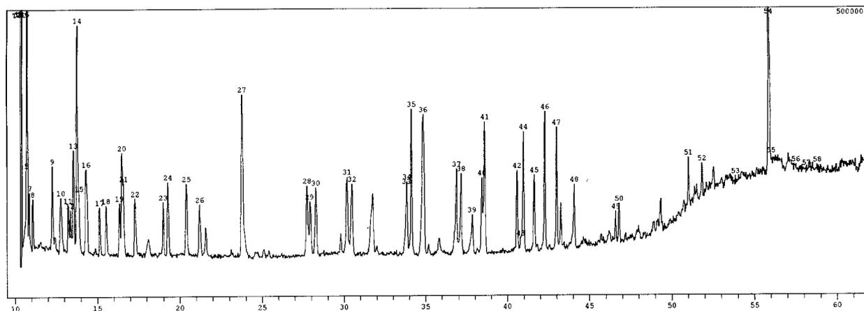
**Figure 2.** Full scan chromatogram of 50 µl of an ethyl acetate standard mixture at the level of 200 pg/µL.
