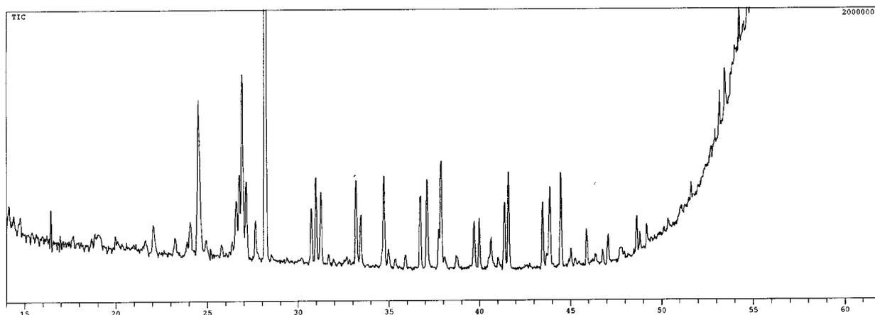
**Figure 4:** On-line SPE–PTV–GC–MS chromatogram of 10 mL of Eindhoven tap water spiked at the level of 1  $\mu\text{g/L}$  using a too long solvent vent time.
