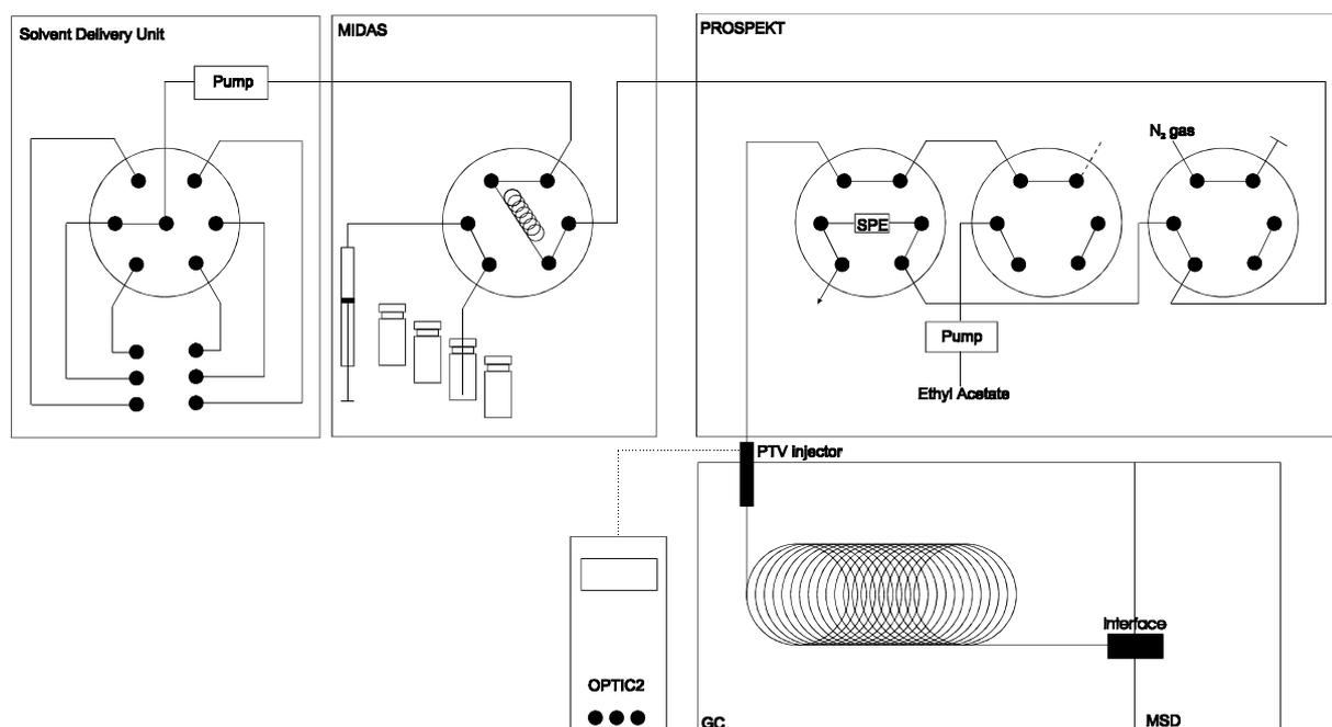
**Figure 1.** Set-up for on-line SPE–PTV–GC–MS.
