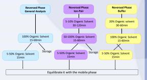
•When the mobile phase does not contain any buffered mobile phases or ion-pairing reagents Use high concentration organic solvent to remove the highly lipophilic contaminants. Increase the content of organic solvent up to 100%. Then, flush the column with 5 column volumes. When observing excessive back pressure, reduce and adjust the flow rate.
