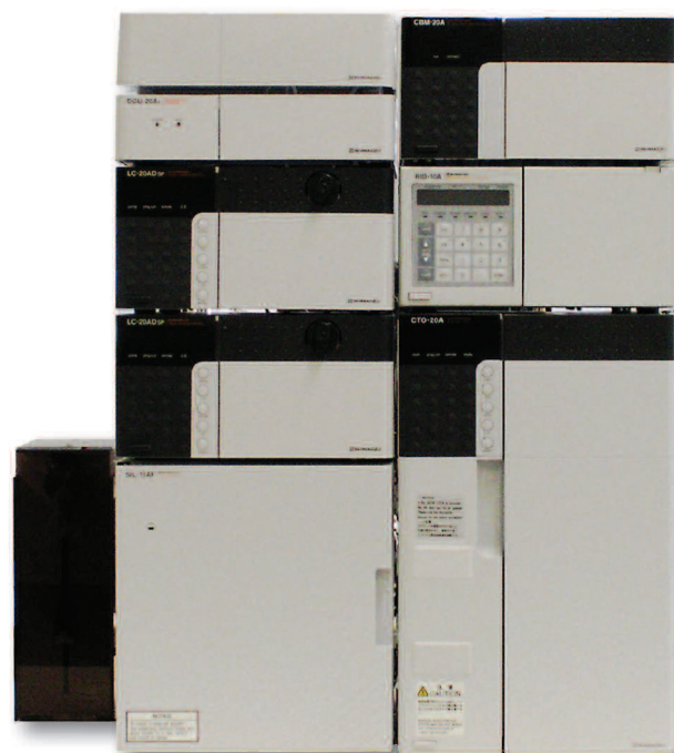
Figure 1: GPC system consisting of HPLC standard components
