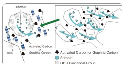
Figure 2. Adsorption on MMSE.
