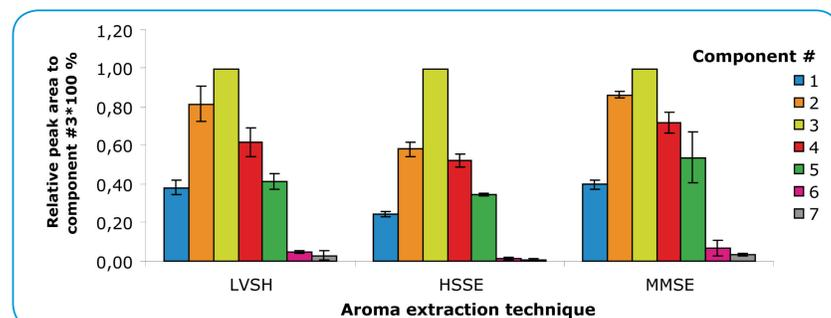
Figure 3. Comparison of the LVSH, HSSE and MMSE technique based on GC/MS analysis. For decoding the components see table 1.
