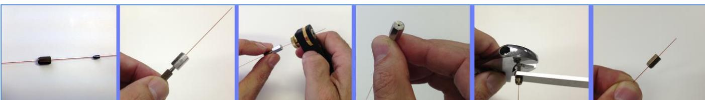
Fig. 4 Column Installation Preparation with Shortix Cutter
