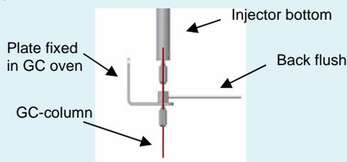
Figure 3: The only difference between normal installation and using the T-joint for back flush is that the column goes through the T-joint to the injector. The original flow path is exactly the same as normal without back-flush. After installation the back-flush is then introduced from the bottom of the injector.
