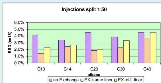
Conditions: alkane mix (12.5 µg/ml); inj. volume 1 µl; liner: DMI liner with cup; OPTIC Temp prog.: start 50°C (10 sec.) to 350°C (rate 10°C/s); Flow: start 100 ml/min (before inj.) then split 1:50; column flow: 1ml/min; column: TC5/MS, 0.25mm x 30m (0.25µm film); Oven prog.: 45°C (2 min hold) to 325°C (rate 30°C/min) hold for 11 min.
