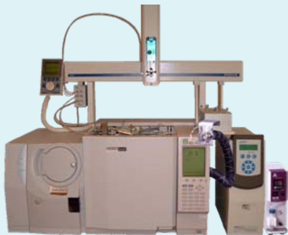
Figure 1: Shimadzu GCMS QP2010, ATAS GL Phaser, Optic 3 and LINEX (LINer EXchanger).
