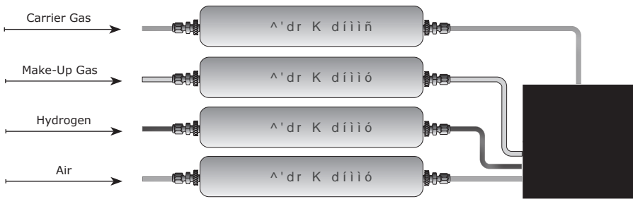
GC/FID Solution 2 (Carrier Gas differs from Make-Up Gas)
